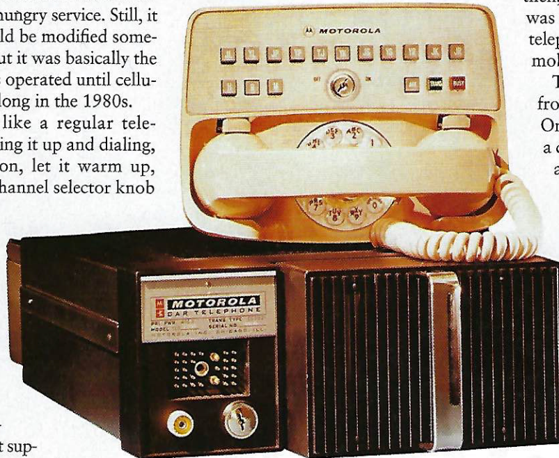
An IMTS car phone, built by Motorola, from 1964. It weighed 40 pounds, half as much as the original 1940s units.
