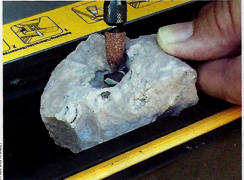
▲ An aluminum oxide grinding stone on my Dremel 952 rotary tool, run at high speed, worked well to separate a garnet from its matrix.
