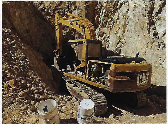
An excavator at the Royal Royston claim removes overburden of rhyolite and kaolin shale to expose the downward-trending turquoise vein.
